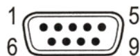
(9-Pin female D subminiature connector as viewed at the end of the cable)
